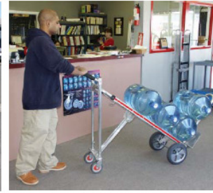
Another type of hand truck converts to four wheels for moving unstable loads.
