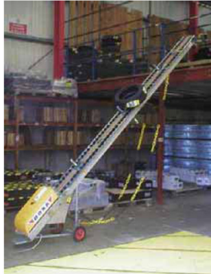
Figure 2. A conveyor used to transport tyres to and from a mezzanine floor store.
