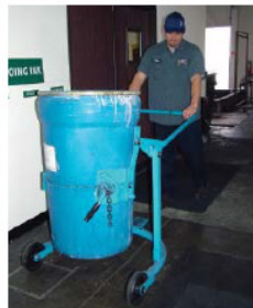
This drum dolly lifts and transports drums.
