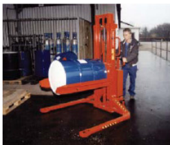
This stacker is well suited for moving loads up to 3,000 pounds for short distances.
