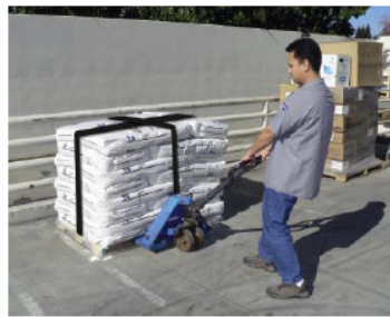
For unstable pallet loads, wrap straps around the load.
