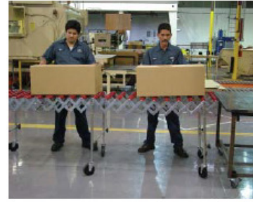
An expandable skate-wheel conveyor is portable and excellent where work needs to have a flexible layout.
