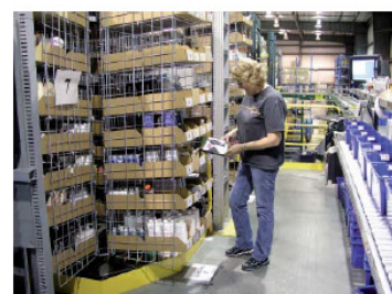
Horizontal carousels rotate and bring items to the worker, eliminating walking and carrying loads.
