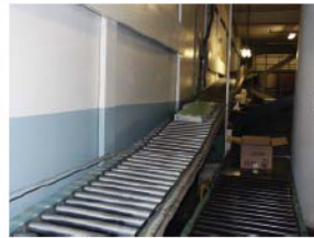
Gravity-activated conveyors work well for short, downhill runs.
