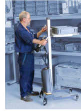
A manually propelled load lifter carries containers. The power lift raises and lowers containers to the appropriate work height.
