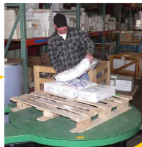
A fixed-height turntable for pallets with short low stacks.
