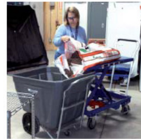
Some industrial tilters can also elevate so that containers or materials being handled are within the worker's power zone.
