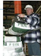
Vacuum lifters can handle sacks and bags that are hard to grip by hand.
