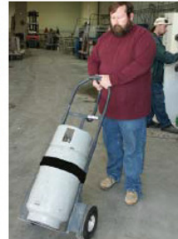
Some hand trucks are specially designed for transporting cylinders.
