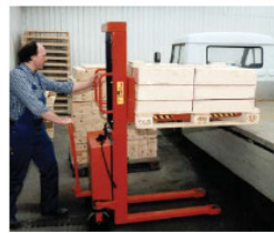
This stacker is well suited for moving loads up to 3,000 pounds for short distances.
