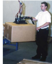
Vacuum lifters make the handling of large or heavy containers easier.
