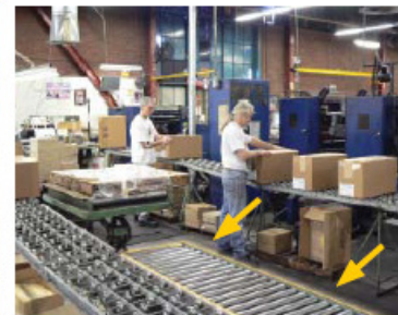
Floor-mounted roller conveyors can handle heavier pallet loads.
