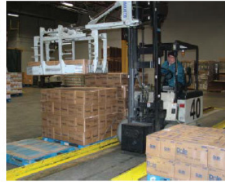
Special attachments are available for removing cartons layer by layer.
