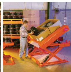
Some industrial tilters can also elevate so that containers or materials being handled are within the worker's power zone.
