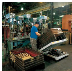
Industrial tilters can improve access to large containers and make handling of materials easier. They can tilt up to 110°, but angles to 45° are most common.
