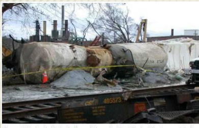
Figure 8. Ruptured chlorine tank car during unloading. The tank has been rotated so that the patched puncture is at the top. Hoses attached to the patch are drawing off chlorine vapors that are then bubbled through a sodium hydroxide solution to reduce their hazard.
